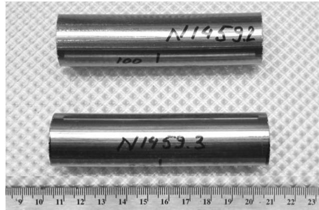
Fig. 1. Two sections of a 25.4-mm-diameter rod extruded from powdered *n*-type PbTe (the scale is graduated in cm).
