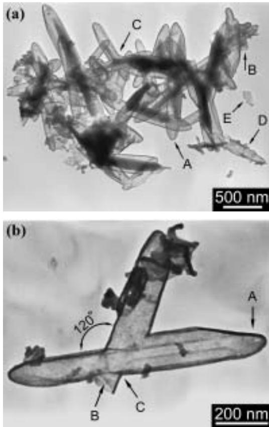
**Figure 3:** TEM images of the  $\text{Bi}_2\text{Te}_3$  nanocapsules hydrothermally synthesized in an opened system at  $65^\circ\text{C}$ , showing closed ends (A), open ends (B), tube branching (C) and sheet segments (D and E).
