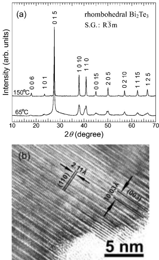
**Figure 1:** The XRD patterns (a) of the hydrothermally synthesized  $\text{Bi}_2\text{Te}_3$  powders with the indexes of the diffraction planes of the  $R\bar{3}m$  phase, and the HRTEM image (b) taking from the  $\langle 1\bar{1}0 \rangle$  direction showing the atomic structure of the  $\text{Bi}_2\text{Te}_3$  powder.
