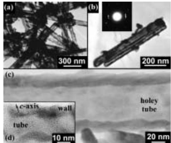
**Figure 2:** TEM and HRTEM images of the  $\text{Bi}_2\text{Te}_3$  nanotubes hydrothermally synthesized in a closed system at  $150^\circ\text{C}$ .
