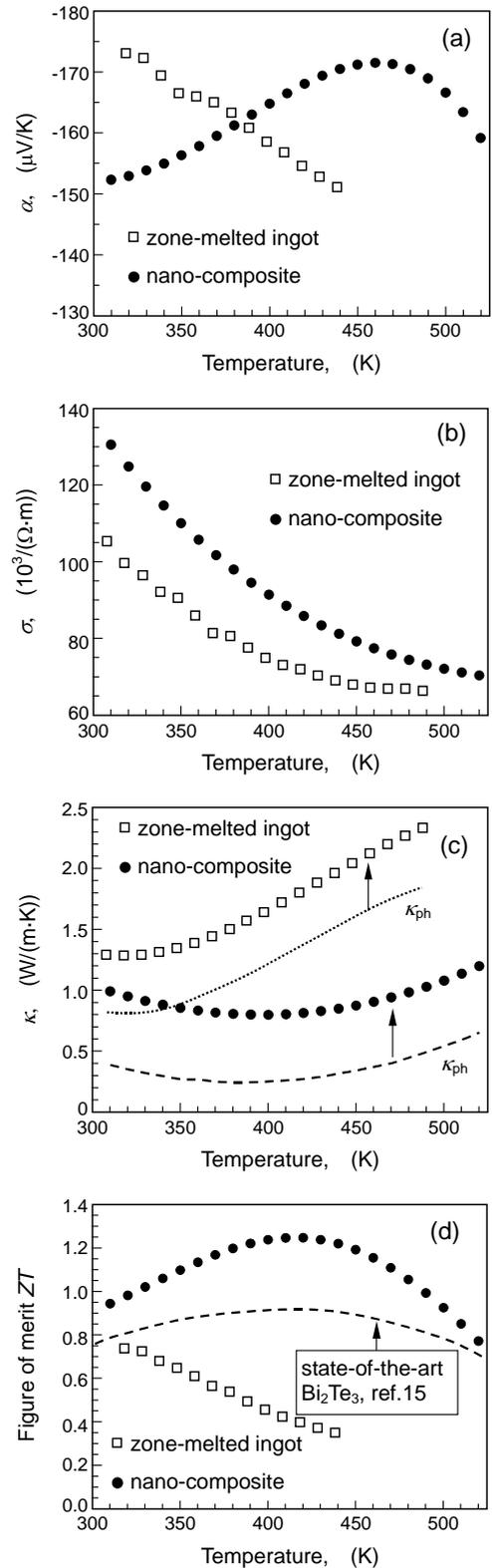
**Figure 4:** Transport properties of the nano-composite sample in comparison with the data measured from the zone-melted sample, for Seebeck coefficient (a), electrical conductivity (b), thermal conductivity (c) and dimensionless figure of merit (d). The lattice thermal conductivities are also plotted in (c) for the zone-melted sample (dotted line) and the nano-composite (dashed line).
