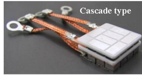
Figure 8: A cascade-type module consisting of Bi-Te and silicide module.
